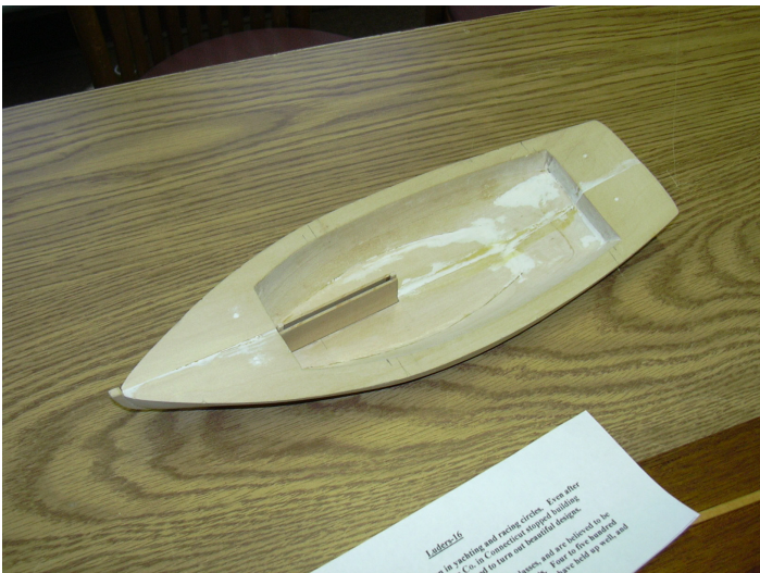
ANOTHER MELONSEED WITH THE CENTERBOARD CASE INSTALLED
